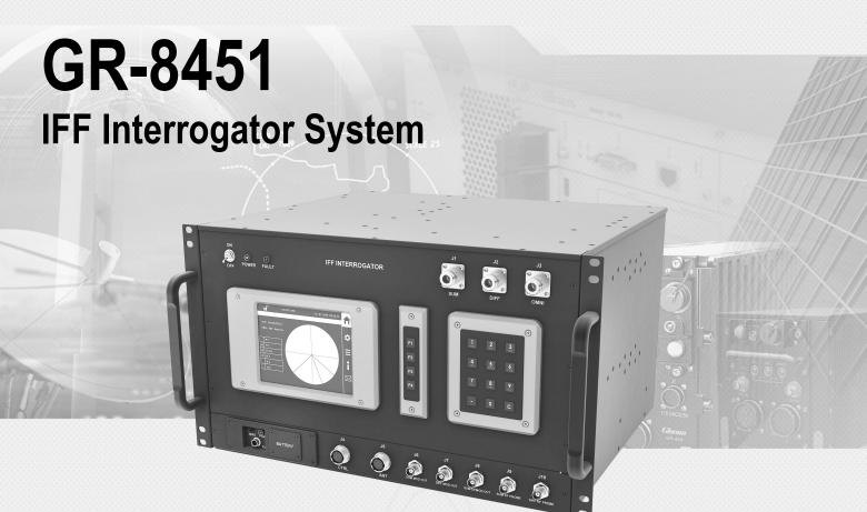
The GR-8451 IFF Interrogator is an advanced long-range IFF interrogator system for the new generation air-defense early warning system. It provides ATCRBS, Mode 4 and Mode S Level 2 aircraft data to the ATC center or weapon system operator.
